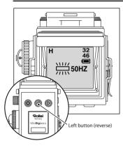
While the camera is in Record mode, press Left button to select frequency for shooting under fluorescent lamp(s). 50Hz and 60HZ alternately appears on the monitor for selection.
